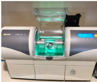
The milling machine used to make crowns using CAD/CAM technology.
